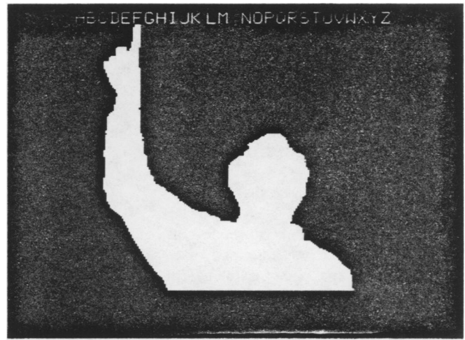
Fig. 7. An experiment in 'typing'; interactive computer environment, 6-ft diagonal video projection screen display; 1985. The participant's image points to a letter causing it to appear as part of a 'typed' message on the screen.
